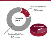
By replacing both heavy hardcore and awkward large insulation sheets, installation time m<sup>2</sup> is approx' 80% faster. Leca® LWA Insulation Fill provides a proven method of providing underfloor thermal insulation replacing both insulation board and hardcore in new-build and refurbishment construction.
