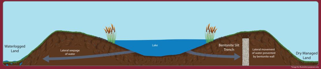
Bentonite granules provide an effective solution to prevent lateral water seepage through natural, and man made bunds and dams. Low permeability vertical barriers can be achieved by cutting a slit trench and simply pouring the granules into the excavation. (or, "sandwich" the granules between geosynthetic (weed) membrane to provide a highly effective clay barrier) Moisture in the ground will cause the granules to swell and form a seal.
