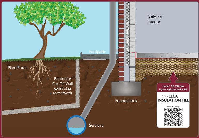
A vertical trench filled with bentonite can be particularly effective to constrain root growth both around newly planted and established trees. Constraint of roots assists the normalisation of matric suction and prevent damage to nearby foundations, service ducts and above ground structures such as road ways, paths and pond integrity.
